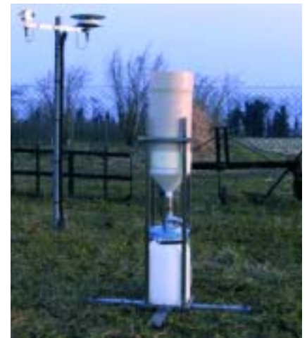
Rain-gauge: used to collect meteoric water samples needed for isotopic analysis.
