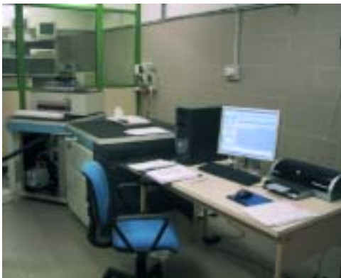
Mass spectrometer: used for oxygen isotopic composition measurement.
